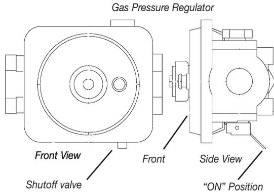
3. Open the manual shutoff valve in the gas supply line. The valve is "open" when the handle is parallel to the gas pipe.
