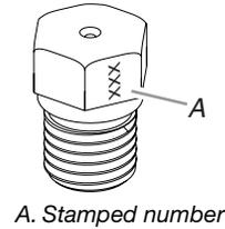
Refer to the following chart for the correct Natural gas orifice spud placement.
