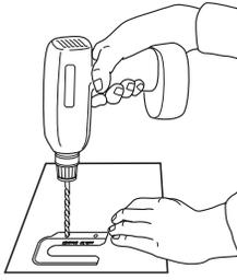
To mount anti-tip bracket to concrete or ceramic floor, use a 3/16" (4.8 mm) masonry drill bit to drill 2 holes at the positions marked on the bracket template. Remove template from floor. Tap plastic anchors into holes with a hammer.
